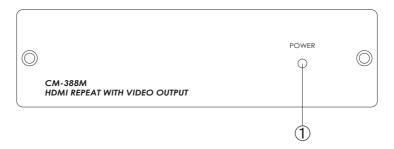
①. Power LED: The LED indicator will illuminate when the unit is connected with power supply.
